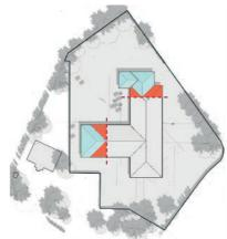
To resolve this the extension was pulled away from the existing building to make room for circulation space with a flat roof designed to float at the level of the existing eaves and a 7° mono pitch roof was then designed as the main roof to the extension to echo the form/ proportions of the existing roof. The pitch has been designed to face inwards, so as to mimic & harmonise with the existing buildings form and enhance the feeling of enclosure within the courtyard.
